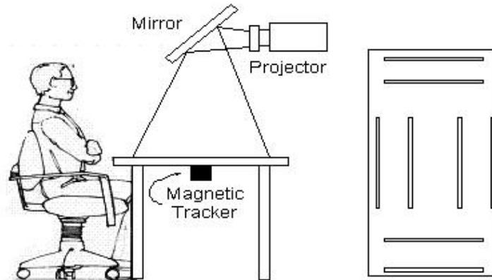
Figure 4.2: The tabletop display is projected onto the surface from above with the Fastrak cube placed underneath the table (left). The force sensing resistors are distributed evenly across the table's surface as seen from the top (right).
