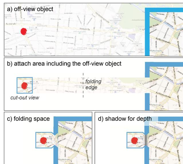
**Figure 2: Canyon attaches a strip of map material containing the object to the view and folds uninteresting space away.**
