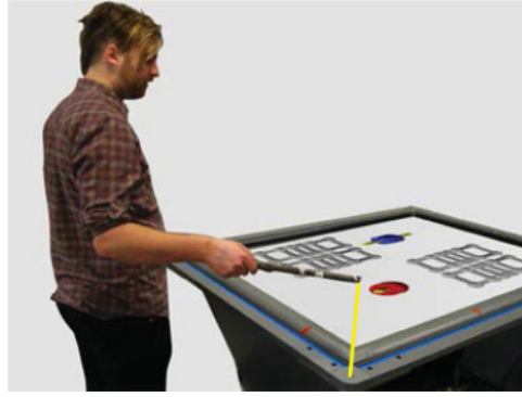
Fig. 15. The participant specified perceived angle by manipulating the angle of a string attached to the right corner of the table and the tip of a wand (string highlighted in yellow). In this simulation, the participant is judging the red and yellow object shown at the quadrant of the surface closest to him.
